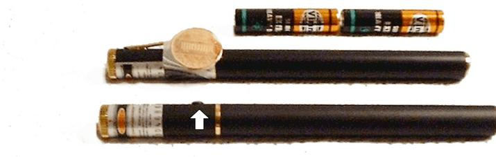
Picture 2: The on-off button is located above the white arrow on the laser pointer in the foreground. The laser behind it has a penny taped over the button for ease of use. These lasers are of equal size, the apparent difference due to the angle of photography. Notice the batteries represent  $\frac{2}{3}$  of the devices length.
